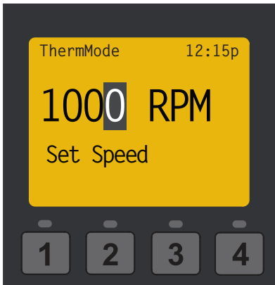
Setting the Thermal Mode Pump Speed
