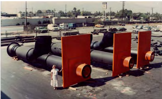
Many, many moons ago... Propeller pumps for an installation in Georgia Sold by General Pump and Machinery, Inc.
