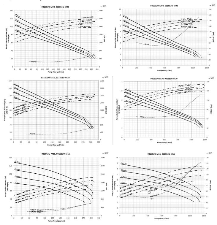
Note: The dashed portion of the pump curves is outside the recommended operating range, and can only be achieved with sufficient NPSHa. Refer to Installation Instructions.
